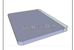
The standard width of a Praxis Elite is 64cm. If this is not wide enough, the table can be optionally expands to 70cm. The length of the table will therefore not change.
