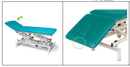
To adjust the head sections pull the control handle, and support the section as it moves. Release the handle to secure the position. The control handle is located under the head section
