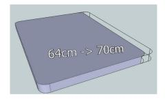
The standard width of a Praxis Elite is 64cm. If this is not wide enough, the table can be optionally expands to 70cm. The length of the table will therefore not change.
